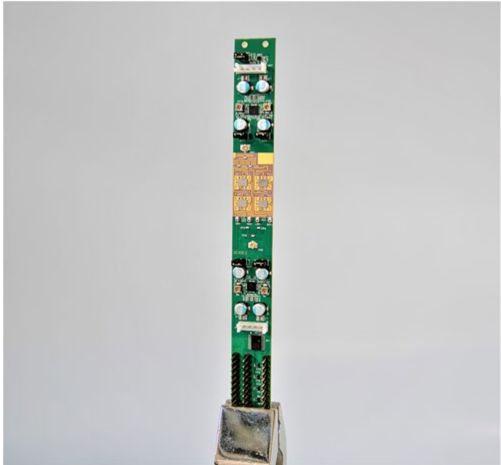
CMOS chips on an 18 mm × 163.5 mm evaluation-board
